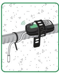
Pour concrete and monitor results in the mobile app or remotely with SmartHub™
